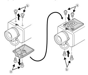
Note: Make sure to use the longer screws @ to secure the bracket.
